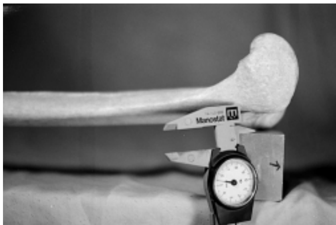
FIG. 4—The distal measure (BDIS) is from the medial patellar surface to the block.
